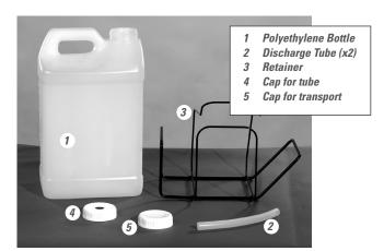
Figure 13—Single polyethylene bottle kit parts
