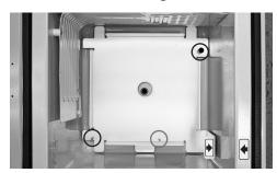
Figure 3—Adapter plate installed (alignment posts circled)
